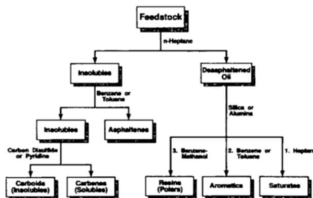
Fig. 5. A general fraction scheme for refinery feedstocks.
